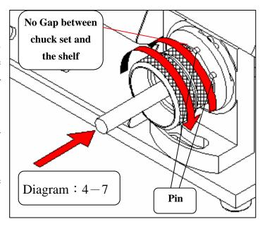
Turn to the other side and grind the drill by the same way. (Diagram 4-7)
