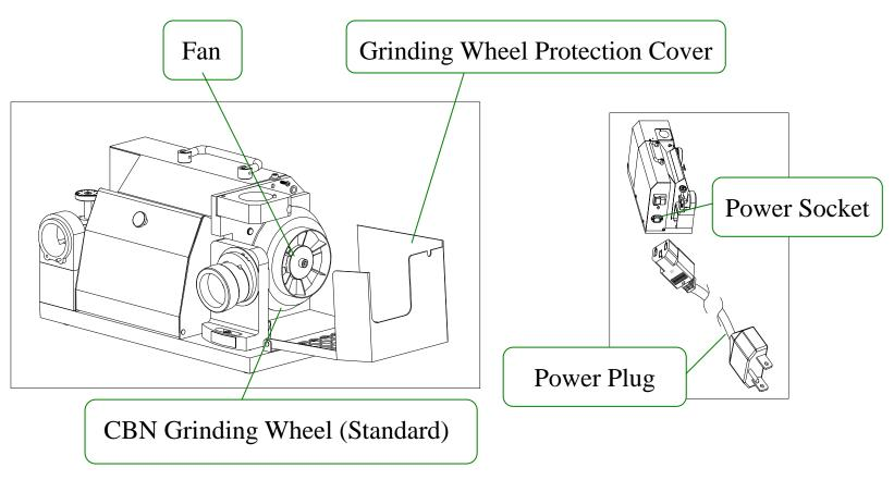
Standard Diameter:  $\varphi$  8mm  $\sim \varphi$  22mm
