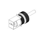
Align the Parallel Devise with the two slots of on the Clamping Nut, then connect them as shown in the left picture.
